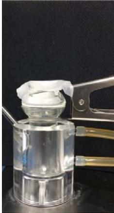
Fig.3: Franz cells from PermeGear (SES GmbH –Analysesysteme, Germany)
